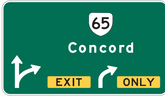
Figure 2E-43. Example of a Partial-Width Overhead Arrow-per-Lane Guide Sign for Intermediate or Minor Interchanges
