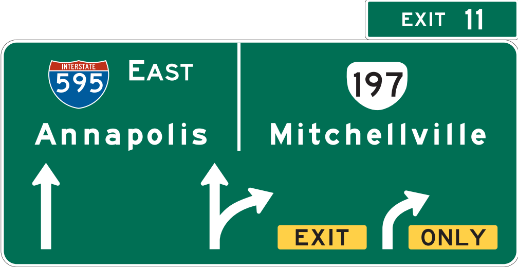
Figure 2E-35. Example of an Overhead Arrow-per-Lane Guide Sign for a Multi-Lane Exit with an Option Lane
